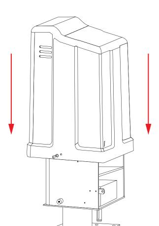
**3. Fasten the housing** to the operator with (2) Washers and (2) Allen Bolts.
